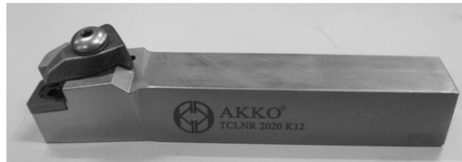
Figure 3. Tool holder of TCLNR 2020K12 [29].
