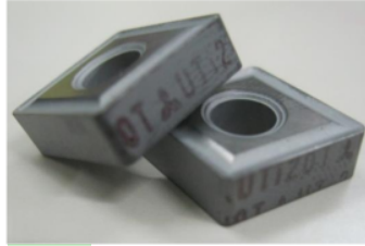
Figure 2. UTi20T Cutting insert [29].
