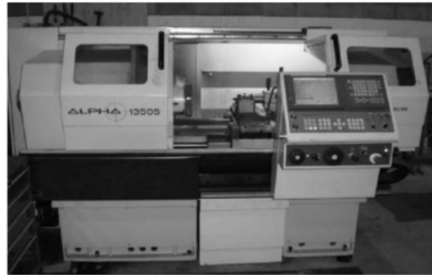
Figure 1. CNC lathe machine with 2 axes, known as ALPHA 1350S.
