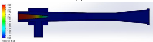
Fig. 6 Pressure contour with the suction diameter ( d=20 mm)
