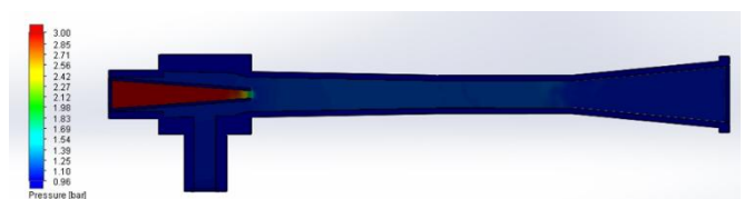
Fig. 4 Pressure contour with the suction diameter ( d=15 mm)
