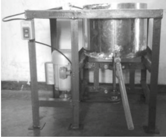
Fig. 1. Spinner machine of cooking oil [4].
