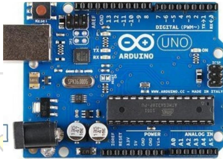
Gambar 2.4 Board Arduino Uno (Sumber: Akbar, 2018)
