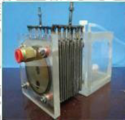
Gambar 2. 4 Generator gas HHO tipe dry cell (Sumber : Sudarmanta bambang dkk, 2016)
