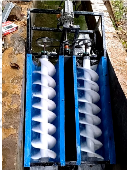
Gambar 7 Pengujiann Turbin Screw
