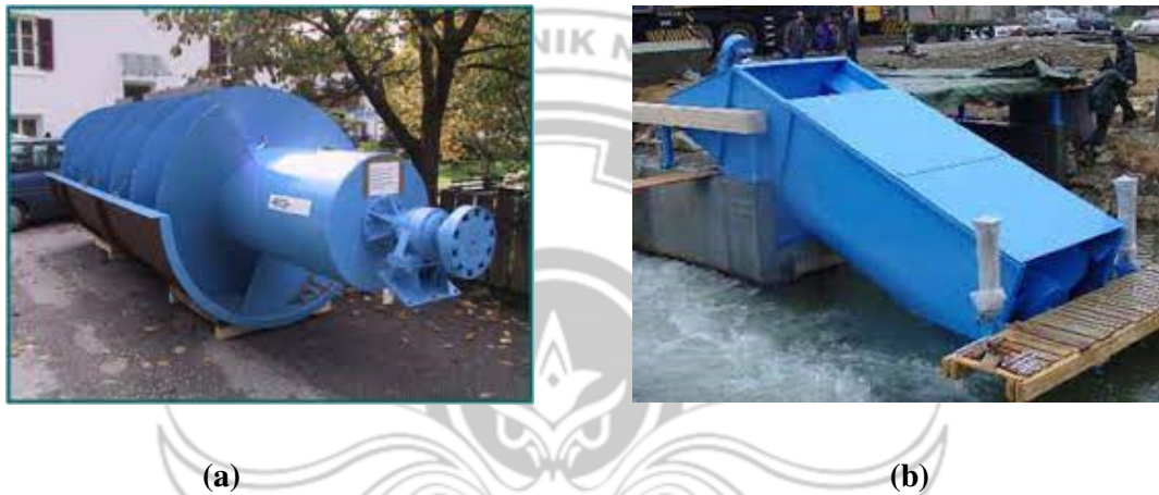
Gambar 2.2 Turbin Screw (a) Tipe Steel Strough (b) Tipe Close Compact
