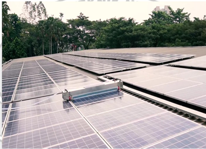
Gambar 2. 2 Solar PV Cleaning Robot
