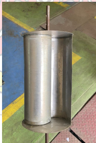
Gambar 4.2 turbin savonius 2 sudu konvensional
