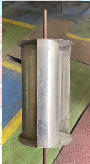
Gambar 4.4 turbin savonius 3 sudu konvensional
