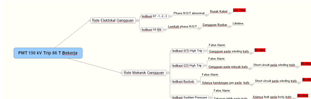
Gambar 4.4 RCPS PMT 150 kV Trip (Sumber: Operator Local Control ULPLTG Tello, 2021)
