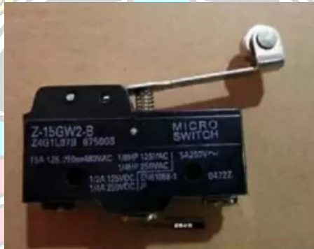
Gambar 2. 9 Limit Switch (Umam, 2019)
