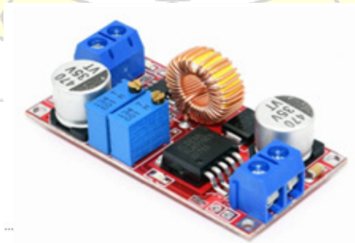
Gambar 2. 8 Converter DC-DC (Hareendran, 2022)
