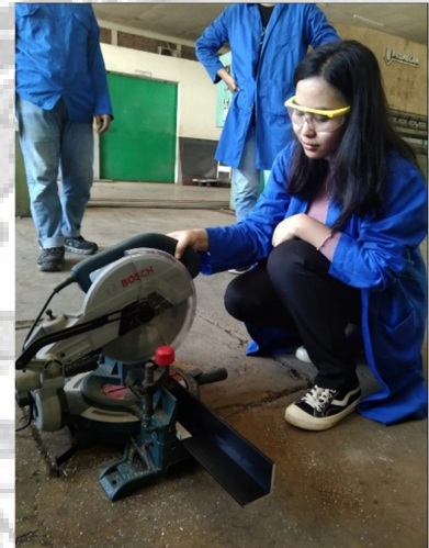
(Proses pemotongan siku Aluminium )
