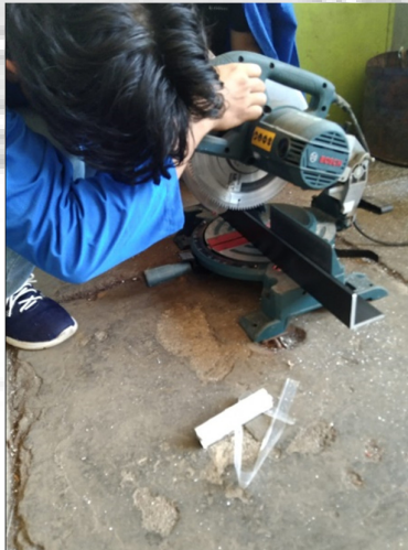
(Proses pemotongan siku Aluminium )
