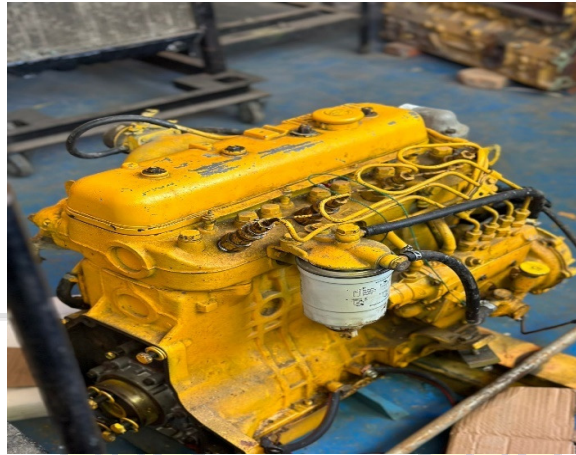
Gambar 2. 1 Engine Daihatsu Taft F50
