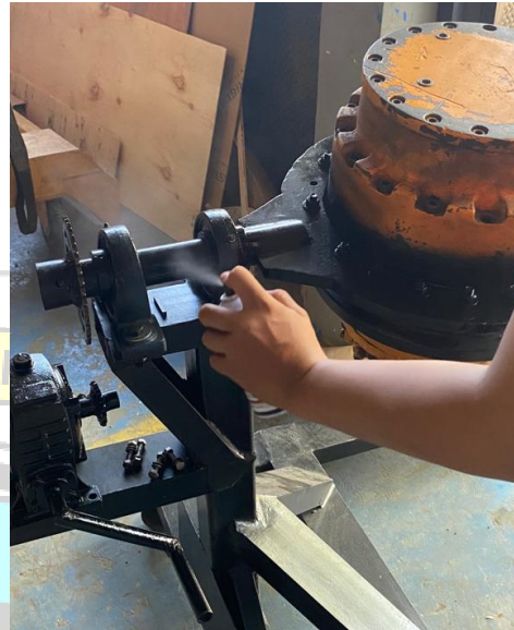
Pengecetan Shaft Final Drive
