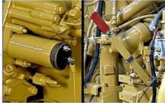
Gambar 2. 10 Fuel Shut Off
