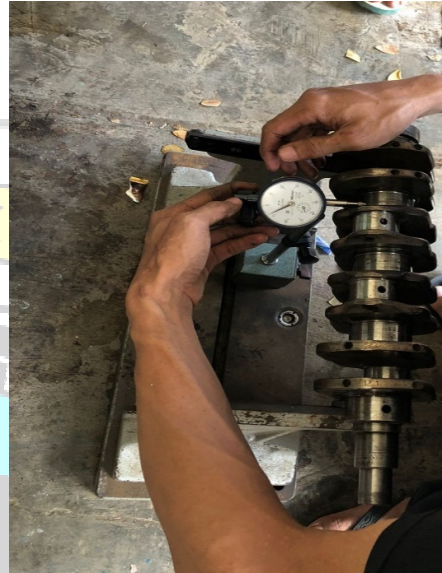
Gambar Pengukuran run out cranshaft
