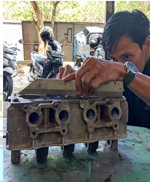
Gambar Pengukuran kerataan Cylinder head
