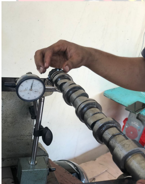
Gambar Pengukuran run out camshaft
