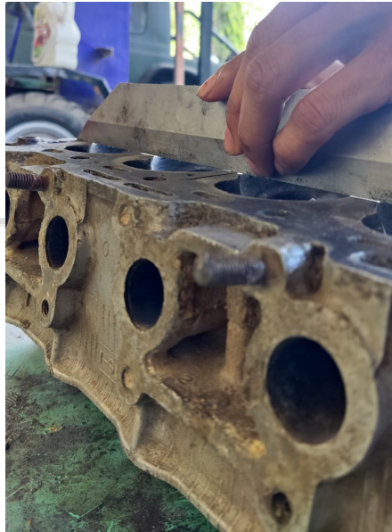
Gambar Pengukuran kerataan Cylinder head
