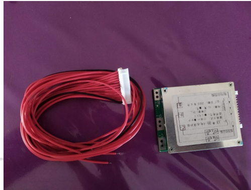
Gambar 2.7 BMS ( Battery Management System )
