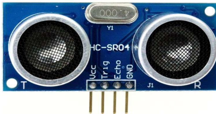
Gambar 2.13, Sensor ultrasonik HC-SR 04
