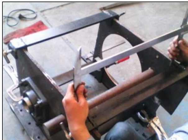
Figure 4. Measurement before welded
