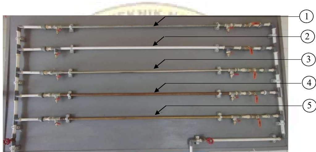
Gambar 4.1 Instalasi pipa alat uji head losses
