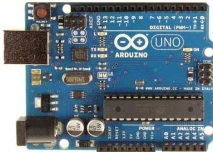
Gambar 2.6 Arduino Uno ( https://www.arduino.cc/en/Products/Counterfeit , 2016)
