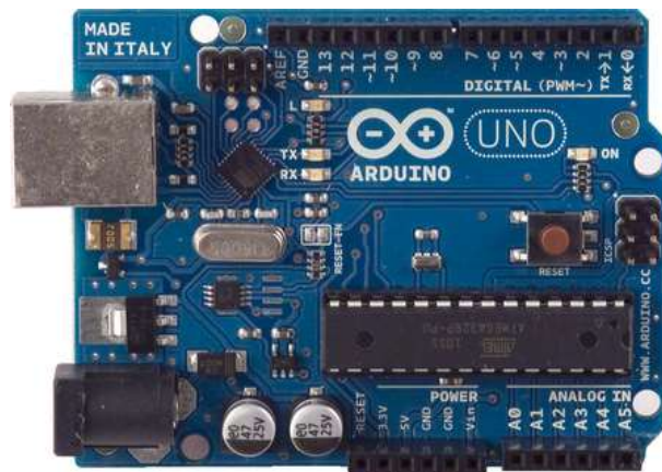
Gambar 7. Board arduino uno
