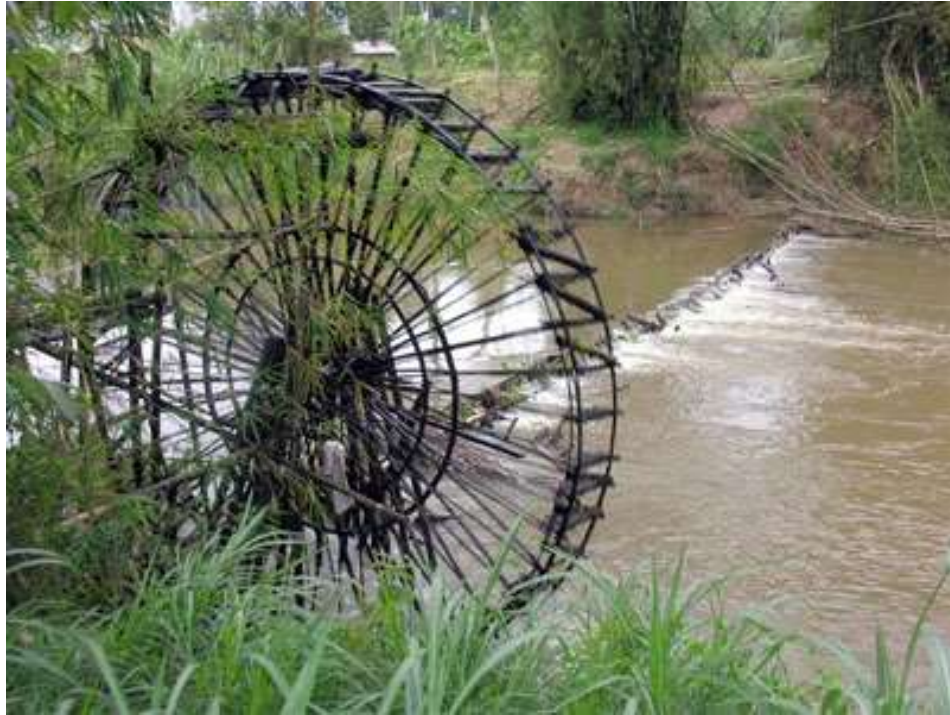
Gambar 2.1 Model kincir air Undershoot Sumber : http://www.melayuonline.com
