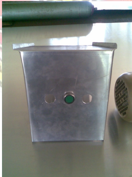
Gambar 6. Panel box kontrol motor.
