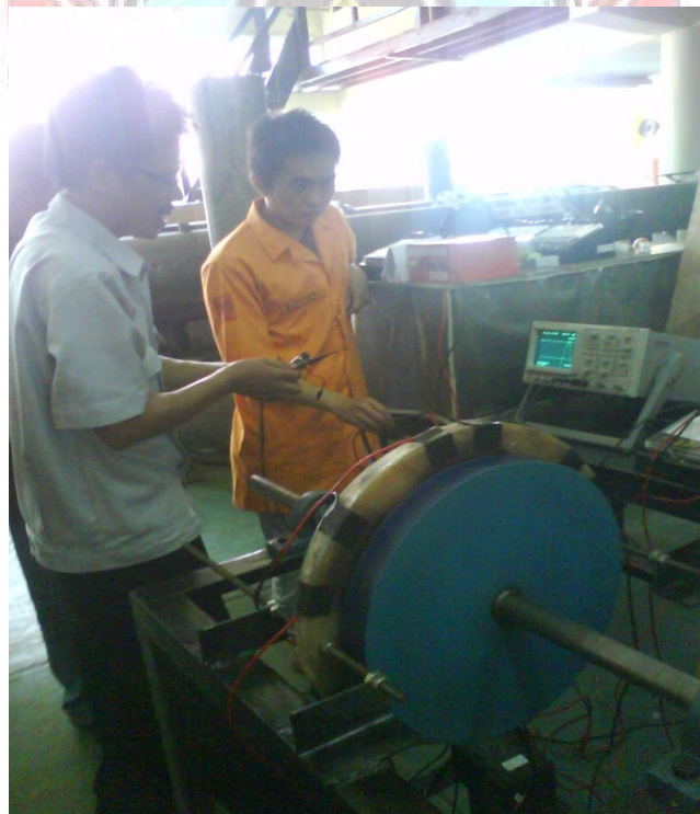
Lampiran 22. Pengujian osiloskop generator fiberglass
