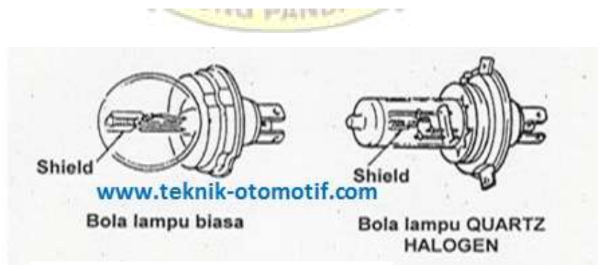
Gambar 2. 7 Lampu Semi Sealed Beam (Sumber : Juan, 2017)
