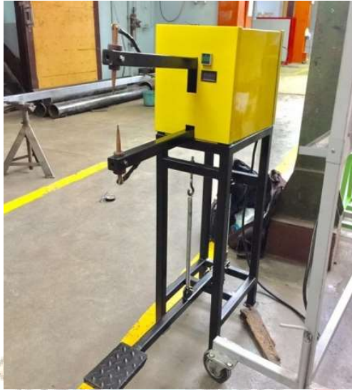
Gambar 2. 5 Spot Welding (Sumber : Tim Website UNY, 2019)
