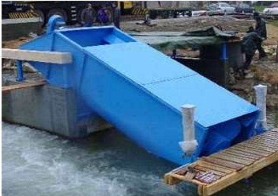
Gambar 2.4 Type Closed Compact Installation (Sumber: www.wikipedia.org/wiki/archimedean_screw )
