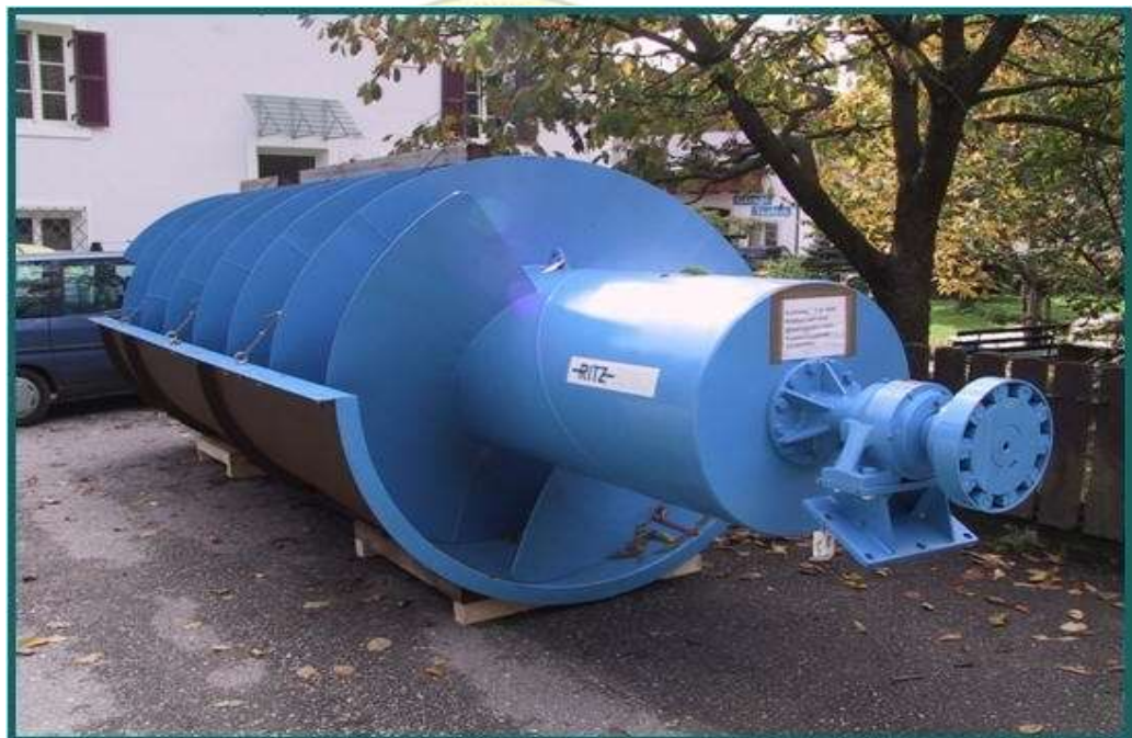
Gambar 2.3 Type Steel trough (Sumber: www.wikipedia.org/wiki/archimedescrow )
