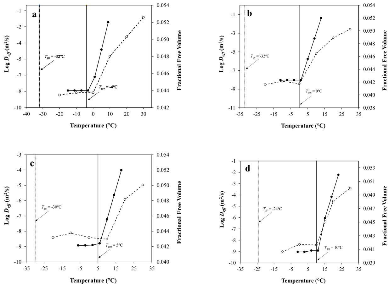
Fig. 8. Effective diffusion coefficient of caffeine (○, left y-axis) and fractional free volume of 2%  $\kappa$ -car/82% PD/1% Cf (●, right y-axis) at (a) 0 (b) 50, c) 100 and (d) 200 mM KCl, with indications of the mechanical and calorimetric glass transition temperatures.
