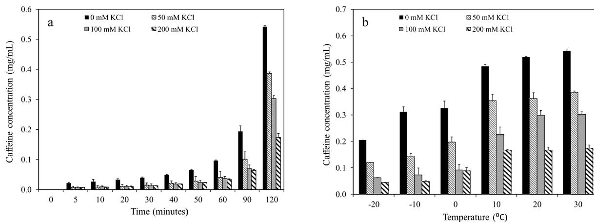
**Fig. 6.** Caffeine release for 2%  $\kappa$ -car/82% PD as function of (a) time at 30  $^{\circ}\text{C}$  and (b) temperature after 120 min.
