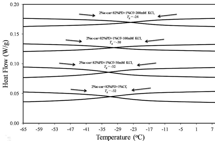
**Fig. 3.** Modulated DSC thermograms of heating and cooling for 2%  $\kappa$ -car/82% PD/1% Cf, 2%  $\kappa$ -car/82% PD/1% Cf/50 mM KCl, 2%  $\kappa$ -car/82% PD/1% Cf/100 mM KCl, 2%  $\kappa$ -car/82% PD/1% Cf/200 mM KCl arranged successively upwards (scanned at a rate of 1 °C/min).
