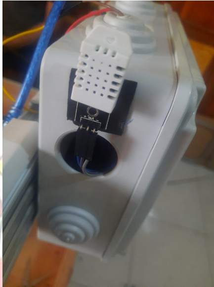
Gambar 4.5 Pengujian Sensor DHT22 di Solar Dryer
