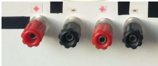
Gambar 4.9 Terminal Input-Output Solar Charge Controller
