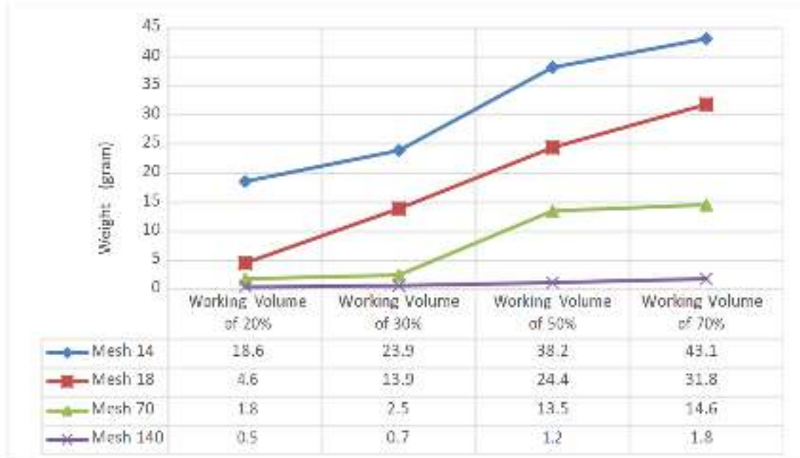
FIGURE 5. The weight of corn cob after 60-minute milling time using 20 mm ball for different of mesh sizes and working volume
