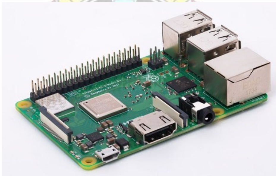
Gambar 2. 4 Tampilan Board Raspberry Pi 3 Model B+ (Sumber: Prastyo, 2016)
