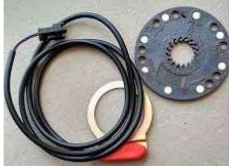
Gambar 2.9 Pedal Assist Sensor
