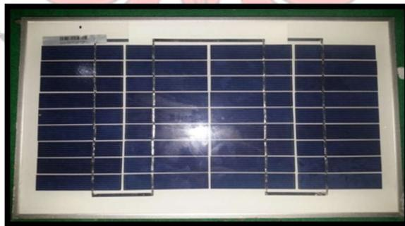
Gambar 2.7. Panel Surya *Polycrystalline*
