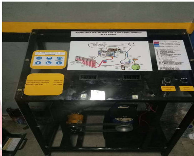
Gambar 4.1 Alat peraga Air Conditioning System
