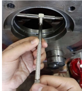
Gambar 3.43 Pengukuran Crankshaft main bearing
