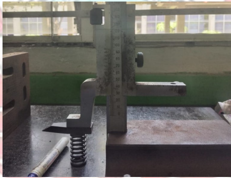
Gambar 3.49 Pengukuran spring valve
