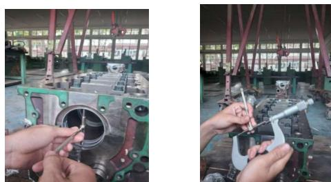
**Gambar 4.7** Pengukuran *Crankshaft main bearing*
