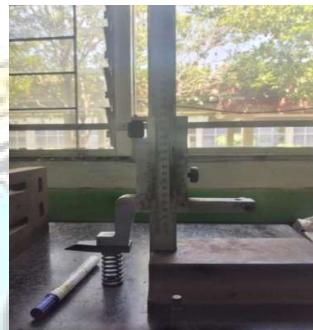
Gambar 4.17 pengukuran *spring valve*
