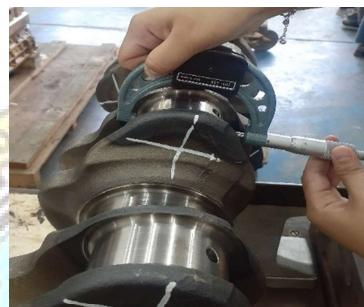
**Gambar 4.3** pengukuran *Crankshaft*
