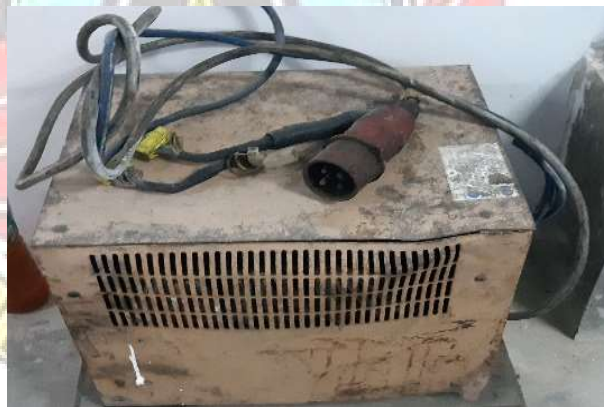
Gambar 2. 7 Charger Baterai Forklift
