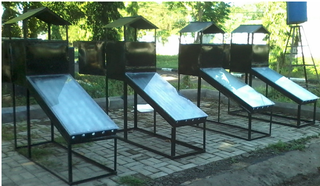
Figure 2: Shelf type of solar dryer with four fin types
