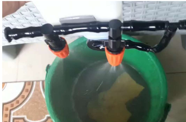
Gambar 3.10 Uji Coba Pompa Wiper 12V
