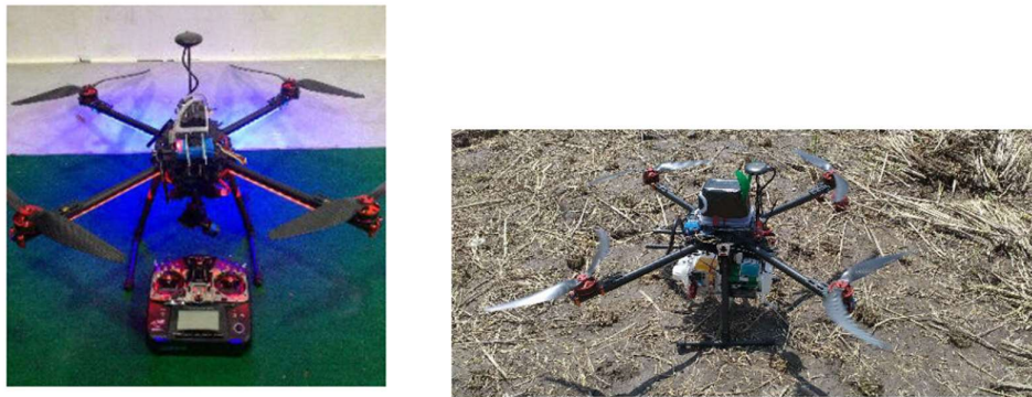
Gambar 2.23 Tabung Semprot Pupuk Cair Berbasis Wahana Quadcopter bagi Lahan Tanaman Padi (Sumber: Akbar dan Anton Yudhana, 2016)
