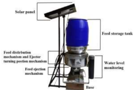
Fig.2. Experimental fish feeding robot prototype with a water level monitoring system developed in this research
