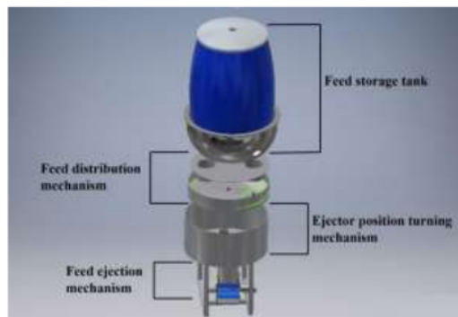
Fig.3. Feed storage tank and the three mechanisms of the fish feeding robot prototype
