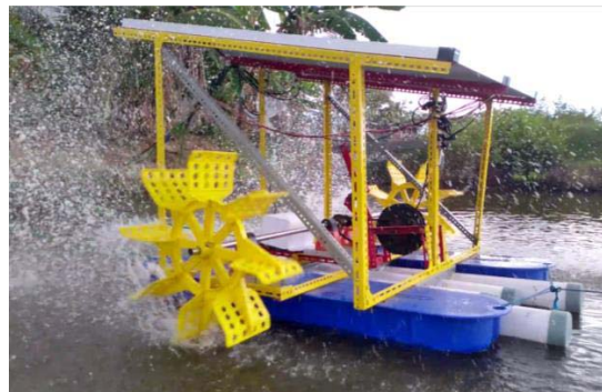
Figure 1. Hybrid Solar-Wind Turbine Paddle Wheel Aerator
