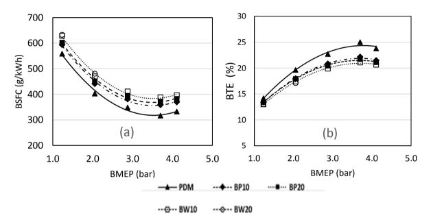
Figure 2 Experiment results for (a) BSFC; and (b) BTE for five fuel tests at 2500 rpm
