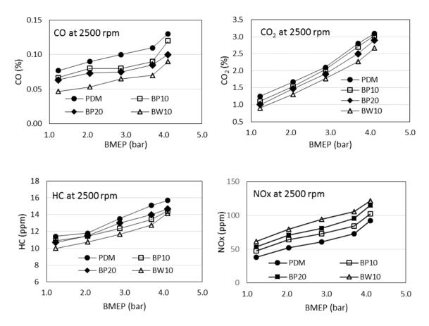
Figure 4 The variation of CO, CO<sub>2</sub>, HC, and NO<sub>x</sub> with engine BMEP at 2500 rpm engine speed
