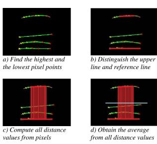
Figure 5. Feature extraction method for a misplaced cap
