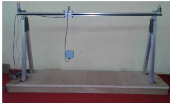
Figure 4. Experimental model of the gantry crane system
