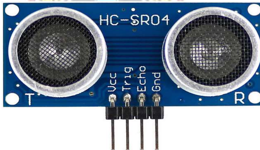
Gambar 2.14 Sensor Ultrasonic HC-SR04
