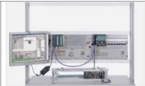
Figure 12. System UniTrain-1 with Profibus Communication
