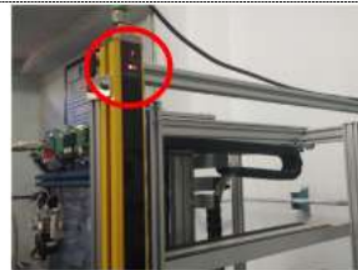
Figure 20. OSSD (Output Signal Switching Device) in the OFF Condition
