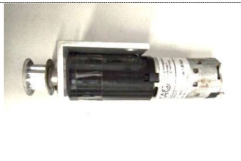
Figure 15. DC motor which has been tensioned between Pulley with Shaft
