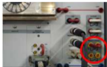
Figure 18. Jumper Safety Fence Panel PLC
