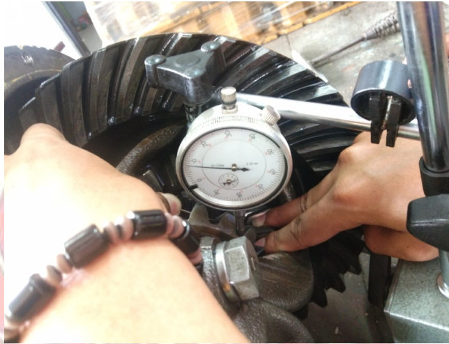
Gambar 4.4 Hasil pengukuran backlash roda gigi samping
