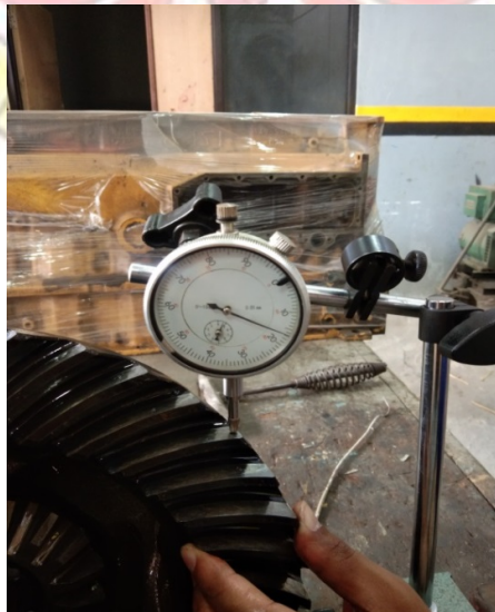
Gambar 4.3 Hasil pengukuran Backlash Ring Gear
