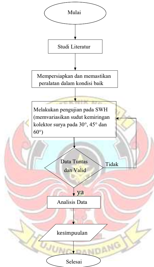
Gambar 3.1 Flowchart Pengujian Solar Water Heater
