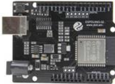
Gambar 2. 4 Mikrokontroler WEMOS D1 R32 Development Board
